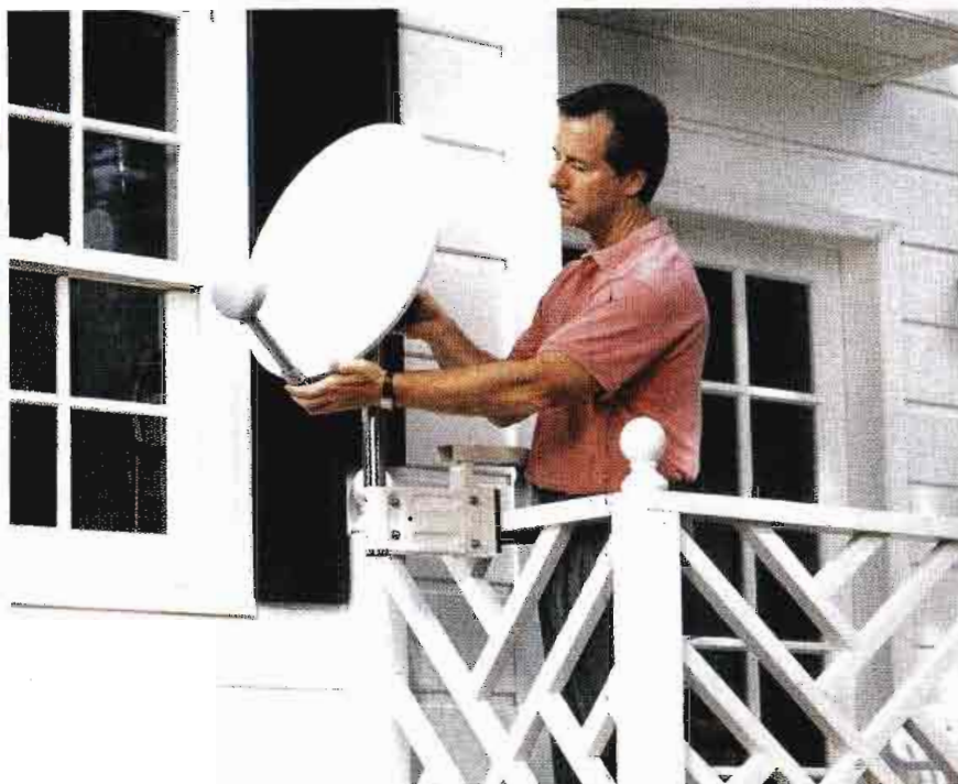
Some see the 18-inch DBS receiving dish as competition to the traditional C-band systems. Others see DBS as a complementary technology.
